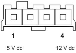
Figure 5-4. 3.5-In. Diskette Drive End of Power Cable
