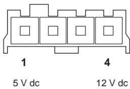
Figure 2-3. 3.5-In. Diskette Drive End of Power Cable
