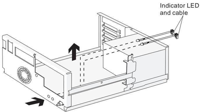
Figure 4-17. Indicator LED and Cable
