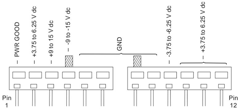
Figure 2-1. System Board Power Supply Connectors (Bottom View)
