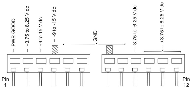
Figure 5-2. System Board Power Supply Connectors (Bottom View)
