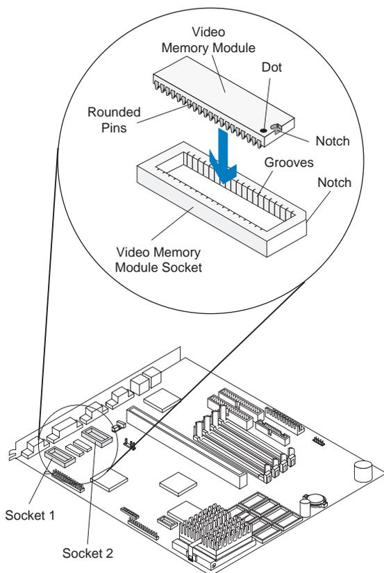
Figure 4-14. System Board Video Memory Module
