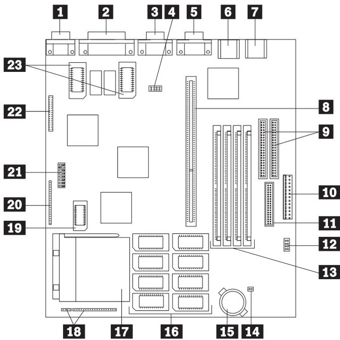
Figure 5-1. System Board Type G-1
