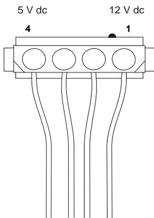
Figure 5-3. Hard Drive or CD-ROM End of Power Cable
