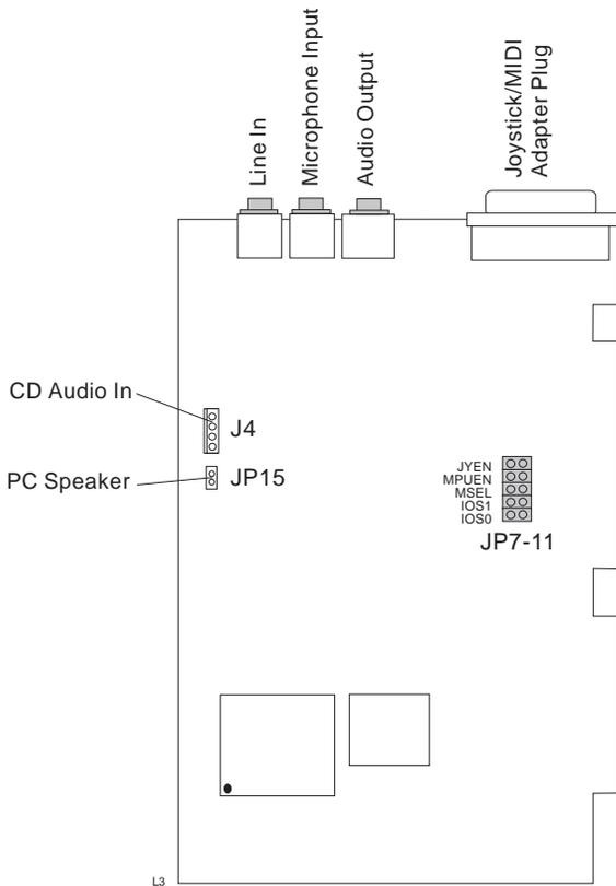
Figure 5-8. CD-ROM Level 3 Sound Adapter Card Jumper Settings
