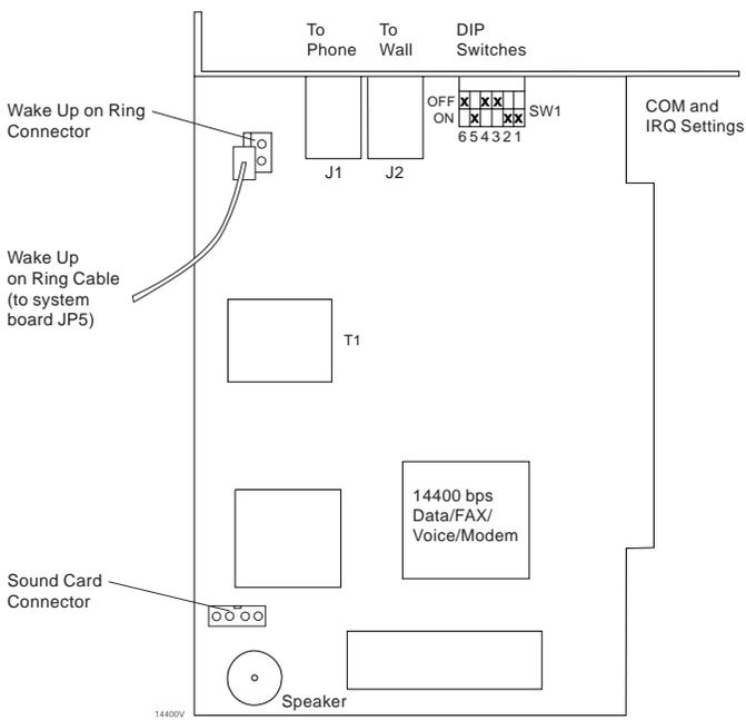
Figure 5-5. 14400 bps Data/FAX/Voice/Modem Adapter Card
