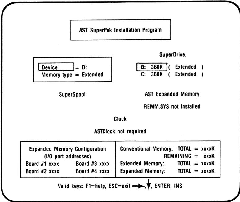
Figure 3-3. INSTALL with SuperDrive Edit Box.
