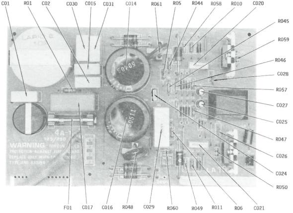
POWER SUPPLY AC INPUT BOARD
