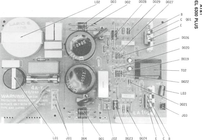
POWER SUPPLY AC INPUT BOARD
