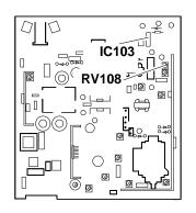
Fig. 3-17 - Frequency adjustment
