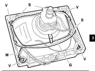
Fig. 3-14 - Position screws securing CRT to video frame
