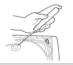
Fig. 3-3 Screwdriver to ground connection
