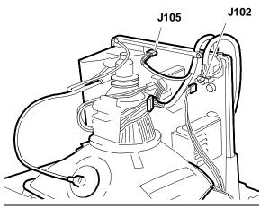
Fig. 3-6 Position of connectors J105 and J102 on the motherboard
