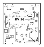
Fig. 3-20 - Distortion (pincushion) adjustment
