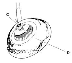
Fig. 3-12 Correct CRT anode fixing
