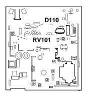
Fig. 3-16 - Voltage adjustment
