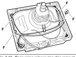
Fig. 3-13 Degaussing coil securing clips removal
