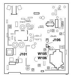
Fig. 3-10 Connector position for connections J101, J106, W105 and W106
