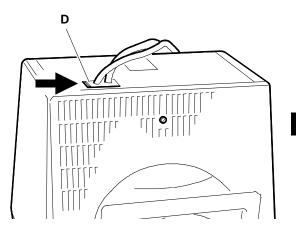
Fig. 3-4 Removing the video cables support
