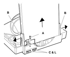
Fig. 3-11 Motherboard removal from video frame
