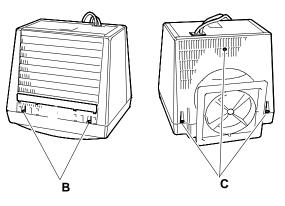
Fig. 3-2 Removal of video casing 5 fixing screws
