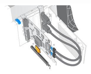
Install a DeckLink PCIe x1 or x4 lane card in a compatible PCI Express slot as shown in the above picture. The DeckLink HD Extreme 2 also has an HDMI bracket, which installs in any spare port, and connects to the rear of the card with the supplied HDMI cables.
