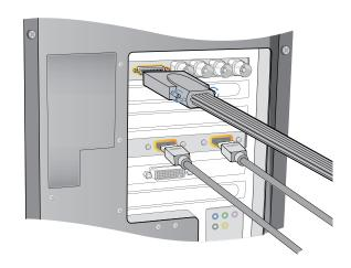
Attach the supplied DeckLink breakout cable to the DeckLink card. The DeckLink HD Extreme 3D card also includes a HDMI bracket as pictured above.
