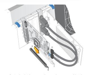
Install a DeckLink PCIe x1 or x4 lane card in a compatible PCI Express slot as shown in the above picture. The DeckLink HD Extreme 3D also has an HDMI bracket, which installs in any spare port, and connects to the rear of the card with the supplied HDMI cables.
