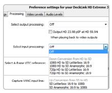
HDTV Up/Down Converter input processing.
