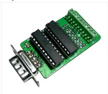
The 80 column output of the Commodore 128 is the same digital RGBI used by the original IBM CGA graphics adapter. Unfortunately nowadays is quite difficult to find a monitor with the suitable RGBI input. The CGA2RGB adapter will convert the TTL RGBI to analog RGB suitable to be connected directly to a 15KHz capable
