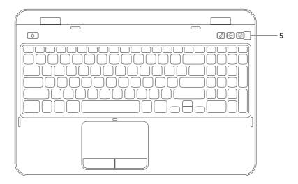
5 Windows Mobility Center button – Press to launch the Windows Mobility Center. Windows Mobility Center provides quick access to your mobile PC settings such as brightness control, volume control, battery status, wireless network and so on.
