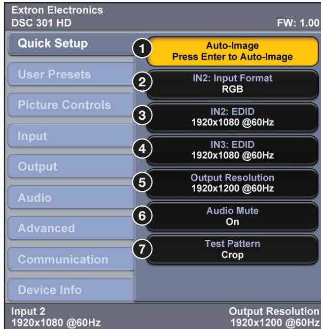
**Figure 4. OSD Menu – Quick Setup Submenu**
