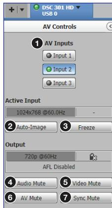
**Figure 34. AV Controls Panel**
