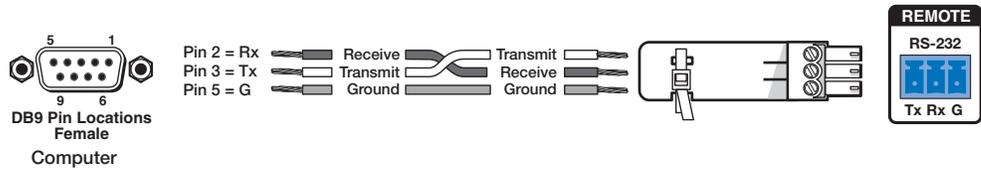
**Figure 2. Wiring the RS-232 Port**
