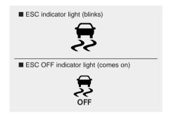
When the ignition switch is placed to the ON position, the ESC indicator light illuminates, then goes off if the ESC system is operating normally.
