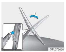
1. Raise the wiper arm and pull out the wiper blade assembly.
