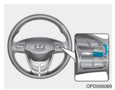
Push the toggle switch up (RES+) and hold it, while monitoring the SET speed on the instrument cluster
