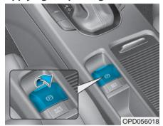
To apply the EPB (Electronic Parking Brake):
