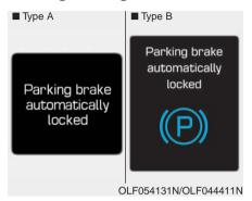
Parking brake automatically locked When the EPB is applied from Auto Hold, a warning will sound and a message will appear.
