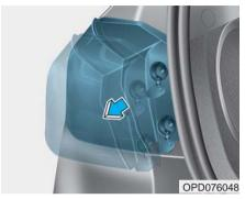
Remove the rear combination lamp assembly from the body of the vehicle.
