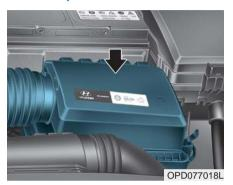
The air cleaner filter can be cleaned for inspection using compressed air. Do not attempt to wash or to rinse it, as water will damage the filter. If soiled, the air cleaner filter must be
