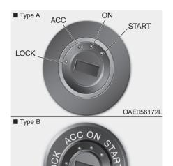
Whenever the front door is opened, the ignition switch will illuminate, provided the ignition switch is not in the ON position. The light will go off immediately when the ignition switch is turned on or go off after about 30 seconds when the door is closed. (if equipped)
