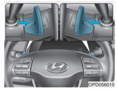
The paddle shifter is functional when the shift lever is in the D (Drive) position or the manual shift mode. With the shift lever in the D position
