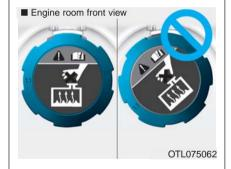
1. Check if the coolant cap label is straight In front.
