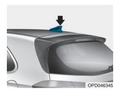
The shark fin antenna will receive the transmitted data (example: AM/FM, SXM signal, GPS).
