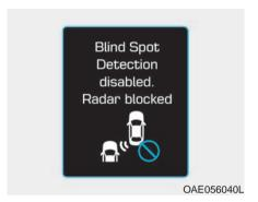
Blind Spot Detection disabled. Radar blocked
