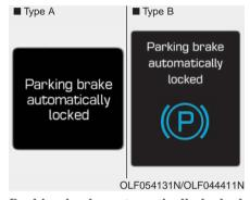
Parking brake automatically locked If the EPB is applied while Auto Hold is activated, a warning will sound and a message will appear.
