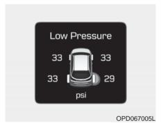
When the tire pressure monitoring system warning indicators are illuminated and the warning message is displayed on the cluster LCD display, one or more of your tires is significantly under-inflated. The LCD position indicator will indicate which tire is significantly under-inflated by illuminating the corresponding position light.
