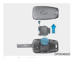
Battery Type: CR2032 To replace the battery:
