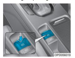
To release the EPB (Electronic Parking Brake), press the EPB switch in the following condition:
