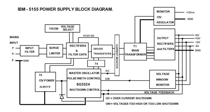
One thing of note is that all switch-mode power supplies have a safety dilemma. This is because the approximately 300V DC power supply is derived from the mains power and is live above ground. This also poses isolation problems of not only for the output supply voltages, but also the electronic sub-circuits in the unit. This problem is solved with isolation transformers which also provide step down functions.
