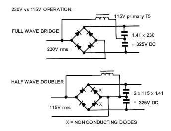
The diagram shows the DC voltage developed across the filter capacitors. In both cases theoretically close to 325V, but in practice with the supply under load it is a little lower at around 312V DC for example with a 230V AC rms input.
