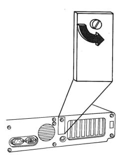
3 Install the battery as shown.
