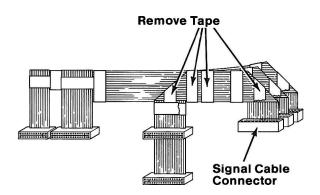
Plug the signal cable (disconnected in Step 5) into the External Diskette Adapter keeping the color stripe to the right, as shown below. Notice that one pin is blank and aligns with the plugged hole in the data cable.
