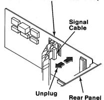
6 Refer to the figure below and remove or carefully cut several bands of tape from the cable assembly to allow the signal cable connector to reach the External Diskette Adapter.
