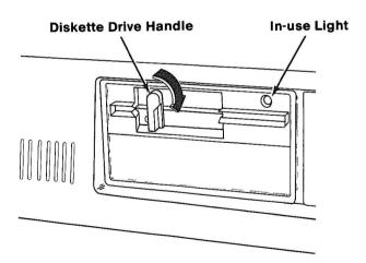
To remove a diskette from the diskette drive, rotate the diskette drive lever counterclockwise and pull your diskette out. Do not remove your diskette when the in-use light is on.
