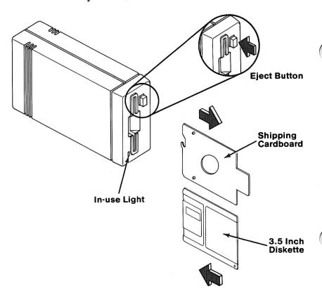
To insert a 3.5 inch diskette, hold it as shown and slide it into the drive until it stops. To remove a diskette, press the eject button.
