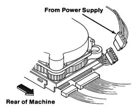
Insert the center connector of the power-split cable into the cable coming from the power supply (disconnected in the previous step). Carefully insert the other wide connector into your fixed disk drive as shown.
