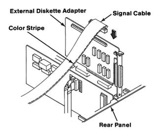
Using the flat cable supplied with this option, connect the Fixed Disk and Diskette Drive Adapter to the External Diskette Adapter, as shown. The flat cable must be installed with the color stripe to the right, as shown.
