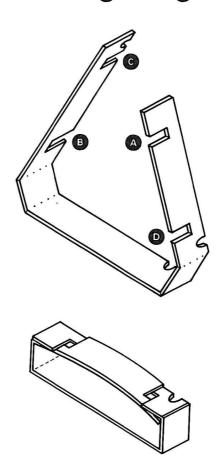
Insert the coprocessor into the safety protector as shown. Make sure that the notch in the safety protector is on the same end as the notch in the coprocessor. The overlapped portions of the safety protector should be on the top of the coprocessor.
