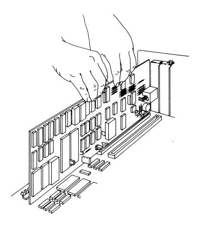
Align the slot in the option retaining bracket with the hole in the rear panel of the system unit (or expansion unit). Start the screw clockwise, then tighten with a flat-blade screwdriver or a 3/16-inch nutdriver.
