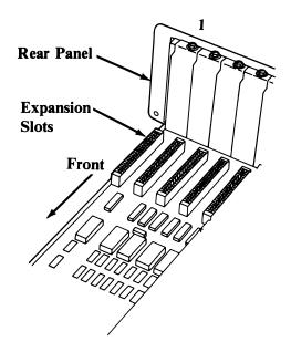
10 Use a flat-blade screwdriver or 3/16-inch nutdriver and remove the screw that holds the expansion-slot cover in place by turning the screw counterclockwise. Save the screw for installation of the option.
