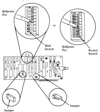
NOTE: Set a rocker switch by pressing the rocker down to the desired position.
