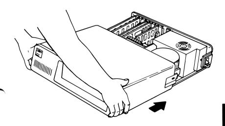
When the cover is all the way to the rear, align the screws with the threaded tabs and tighten.
