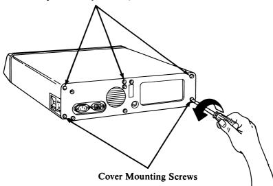
8 Carefully slide the unit's cover away from the rear and to the front, as shown in the figure below. When the cover will go no further, tilt it up, remove it from the base, and set it aside.
