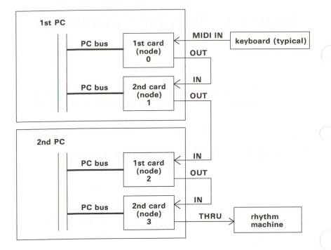
Figure 9-1. Connections of Multiple Cards and External MIDI Devices
