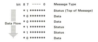
Figure 3-2. Data Flow with Status Byte Control
