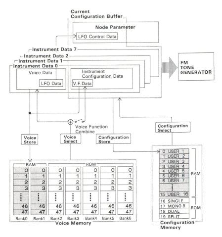
Figure 1-4. Block Diagram of the Sound Processor
