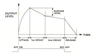
Figure 8-4. Parameters Programmed for the Envelope
