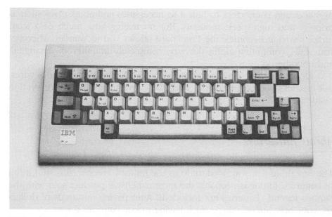
IBM redesigned its PC*jr* keyboard to resemble that of the PC and PC-XT. Both this keyboard and the original Freeboard can transmit keystrokes to the PC*jr* using infrared signals rather than a cord.
