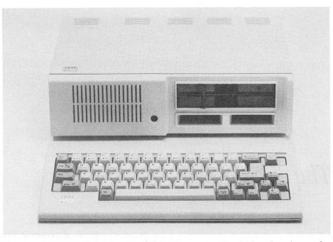
The new PCjr, with its attractive, full-travel typewriterlike keyboard and its 360K disk drive.
