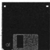
Many PCjr users confuse a hard drive with a hard jacket 3 1/2 inch diskette. A 3 1/2 inch diskette is actually a floppy disk in a hard plastic jacket. A hard drive can not be removed from the computer. For this reason, a hard drive is also referred to as a fixed disk.
