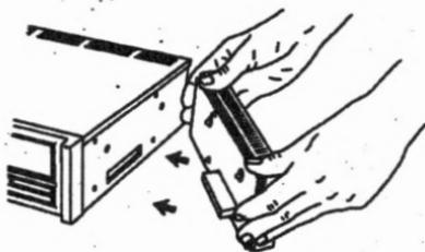
Next, position the sidecar so that it aligns with the rectangular cutout, then press the sidecar in place. Four screws are provided to keep the sidecar from coming off.
