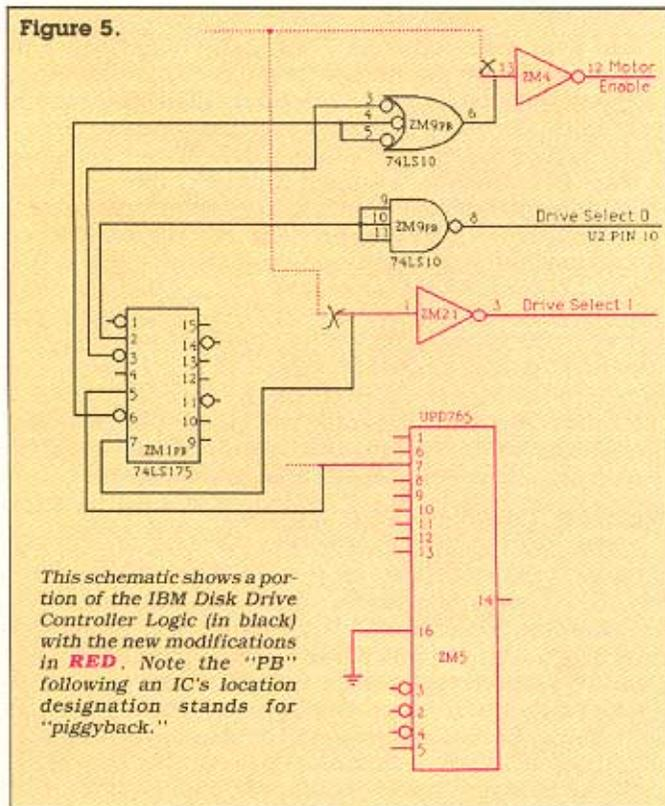
This schematic shows a portion of the IBM Disk Drive Controller Logic (in black) with the new modifications in RED. Note the "PB" following an IC's location designation stands for "piggyback."
