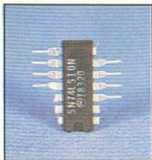
RIGHT: The prepared "piggyback" IC for location ZM1 (74LS175) is shown here after its pins have been formed (or removed) per the instructions in the text.
