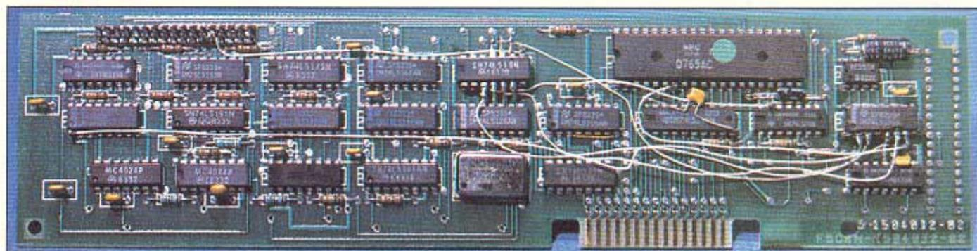
The completed project with the modified controller board and new cable installed prior to "buttoning up."
