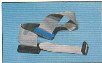
Shown above is the new cable that connects the modified controller board to the two disk drives (the original drive inside the PCjr and the additional drive on the outside). The portion between the controller board connector and the internal drive has been sized and formed to match the original IBM cable.
