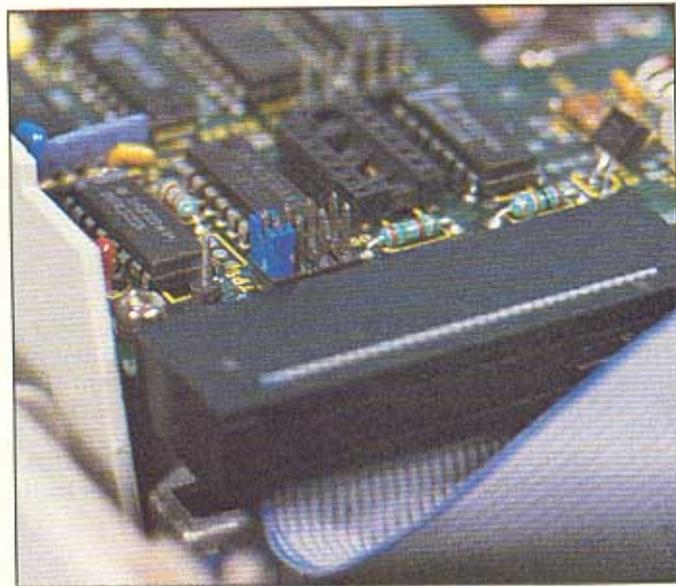
(coming out of the PCjr) onto this edge-type connector. Plug in the power on the new drive and turn on its power switch. If the red light of the new drive comes on and stays on, the flat cable connector is upside down. Turn off the power of the second drive, reverse the flat cable connector at the new drive end, and try again. The red light should not come on. Finally, replace the external disk drive's cover while guiding the new cable out the unit's cable slot.
