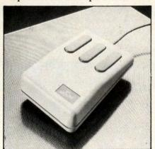
word processing programs for use with this keyboard substitute, including VisiCalc, MultiPlan, and pfs:write. You can also create your own mouse-accessible menus for other PC and PCjr programs. The optical PC Mouse comes with a light-reflecting pad that monitors the mouse's movements and its own power supply. It costs \$295. It connects to the PC or the PCjr with a standard RS-232C interface. Contact: Mouse
