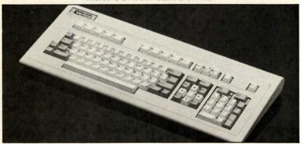
Key Tronic Corporation has come out with a replacement keyboard for the PCjr, which features separate cursor-control keys; a numeric pad; function keys across the top; and a cable connection. Its 99 keys, with the characters marked on top, are in the familiar typewriter placement; the function keys come with removable templates. Model KB5151 *jr* lists for \$255, and is available from Key Tronic Corporation, Dept. PM, P.O. Box 14687, Spokane, WA 99214, (509) 928-8000.
