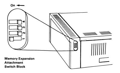
c. With 128KB memory installed inside your IBM PC*jr*, set the 128KB Memory Expansion Attachment switches as shown below:
