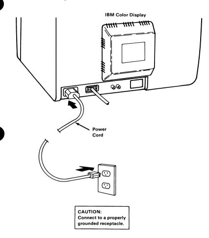
Plug the IBM PCjr and all option Power cords into wall outlets.
