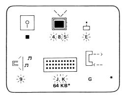
The advanced-test menu consists of symbols, with each symbol representing one area of the IBM PCjr. The letters or numbers below the symbols are IDs of tests you can perform.
