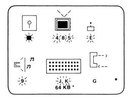
The IDs for joystick and sound always blink because their interfaces are on the system board. The blinking does NOT mean a joystick or external speaker is installed.
