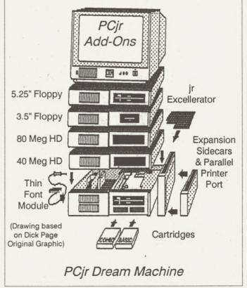
Meg of RAM, two 5 1/4 inch disk drives, a 3 1/2 inch disk drive, two hard drives, a 9.54 MHz speedup board, speech attachments, and a 2400 baud modem, and a Thin Font Module -- all attached to your PCjr and powered by a 150 watt power supply.
