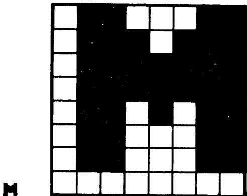
Normal PCjr characters are two dots wide. While two-dot-wide characters are sharp and distinct in 40 column modes they tend to "fill in" or "close up" when you switch to an 80 column mode. And when two fuzzy characters are displayed side by side things get much worse, and the characters tend to blur together.
