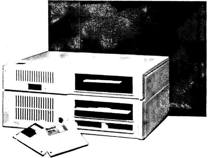
The disk drive that came with your PCjr uses 5 1/4 inch flexible diskettes. These diskettes can be formatted by DOS to have 40 tracks on each side - enough room for 360K of information.
