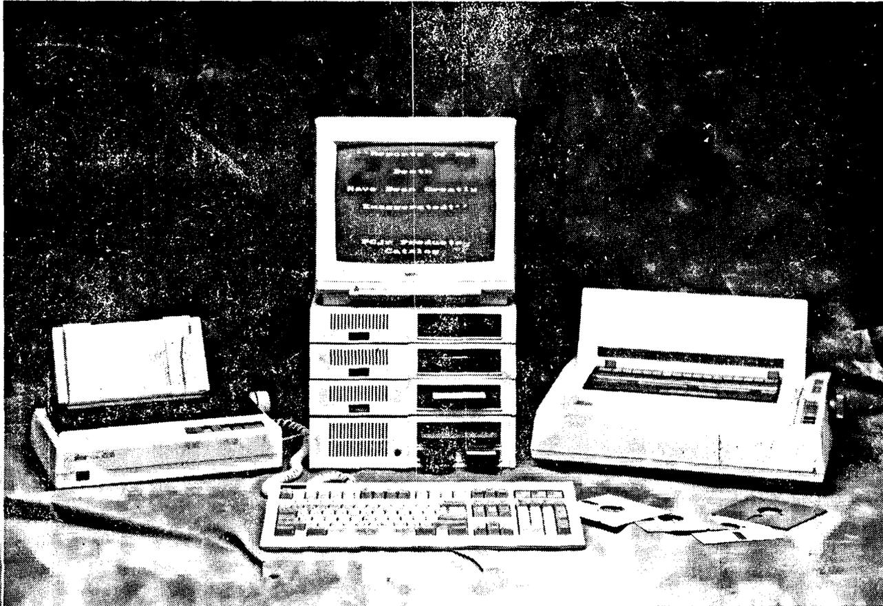
*Featured in photo: PCjr with one 360K diskette drive for PC compatibility, one 3 1/2 inch diskette drive for PS/2 compatibility, one 1.2 MB diskette drive for PC-AT compatibility, and one 20 MB hard disk drive. Also shown, Magnavox CM8762 RGB monitor, Star NX-1000 dot matrix printer for fast yet economical printing, NEC elf 370 Spinwriter printer for true letter quality printing, and Datadesk 101 keyboard. The PCjr is powered by the 150 watt Junior Drive power supply.*
