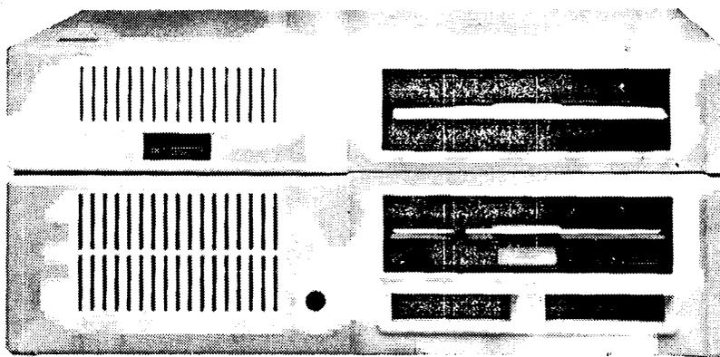
The Enhanced model of the PCjr only comes with one disk drive. At times this can be quite inconvenient. Because most serious software packages are designed to run on systems which have two drives. And because backing up diskettes with only one disk drive can involve a lot of disk swapping.
