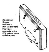
Allows you to connect most printers that have an industry standard parallel interface to the PCir. Installs on the side of the PCjr without special tools or skills.
