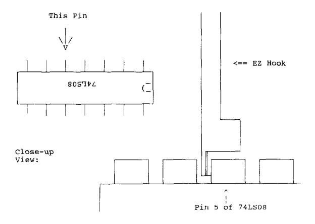
The EZ-Hook is attached by first exposing the metal hook. This is done by compressing the EZ-Hook's main body:
