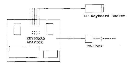
10. Place the Internal Keyboard Adapter in the same location that the IR module was taken from. Align the 8 pin connector with the 8 pin socket located about 1/2" behind the two plastic posts that held the IR module in place, and firmly press the Internal Keyboard Adapter down until both posts have snapped into the mounting holes.
