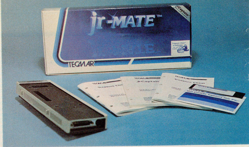
Photo 1: The Tecmar jrCaptain peripheral comes with three manuals, a diskette of software programs, its own power source (the small transformer is not shown here), and the special screws to mount it to the PCjr.
