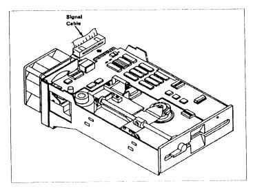
Ok, job well done, now make the quick test. Sit the drive into the junior without snapping in the mounting feet. Plug in the power cord and video cable. Turn on the machine, the IBM LOGO should appear just as before. GREAT, turn the machine off and unplug it again.
