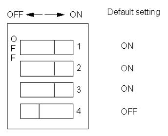
*Note:* When a drive 1 (slave) is installed in the system with a drive 0 (master) already installed, there is no change to the switch setting for a drive 0 (master). Only the switch of drive 1 (slave) is required to be set.
