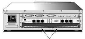
If the bottom slot of your chassis has two separate shielding strips, you will need the field upgrade kit in order to install an extended-format module in the bottom slot of the chassis.
