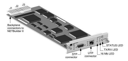
**LEDs** The Token Ring+ module has three LEDs for displaying information. Table 2-3 describes each of the LEDs.
