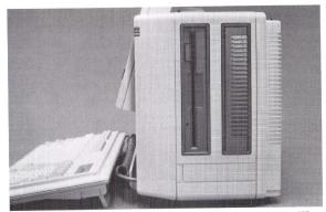
Figure 2-7. Drive Positions on the COMPAQ PORTABLE III Personal Computer.
