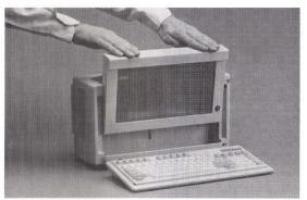
Figure 4-1. Lowering the COMPAQ Dual-Mode Plasma Display.
