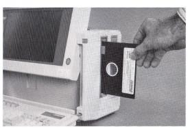
Figure 2-11. Inserting a Diskette into the Diskette Drive.
