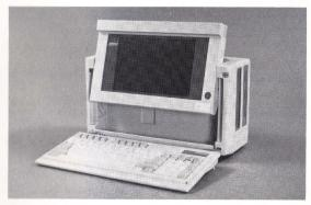
Figure 6-1. COMPAQ Dual-Mode Plasma Display.
