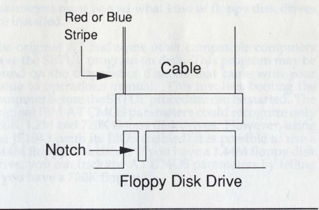
WARNING! Connecting this cable backwards may cause irreversible damage!
