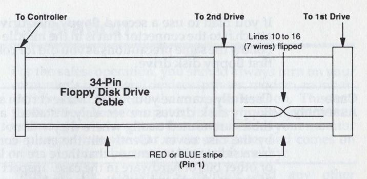
Attach the end of the cable to the first floppy disk drive (drive A:). Make sure the it attaches to the connector on the end of the cable and that the red or blue stripe on the cable faces the correct direction.
