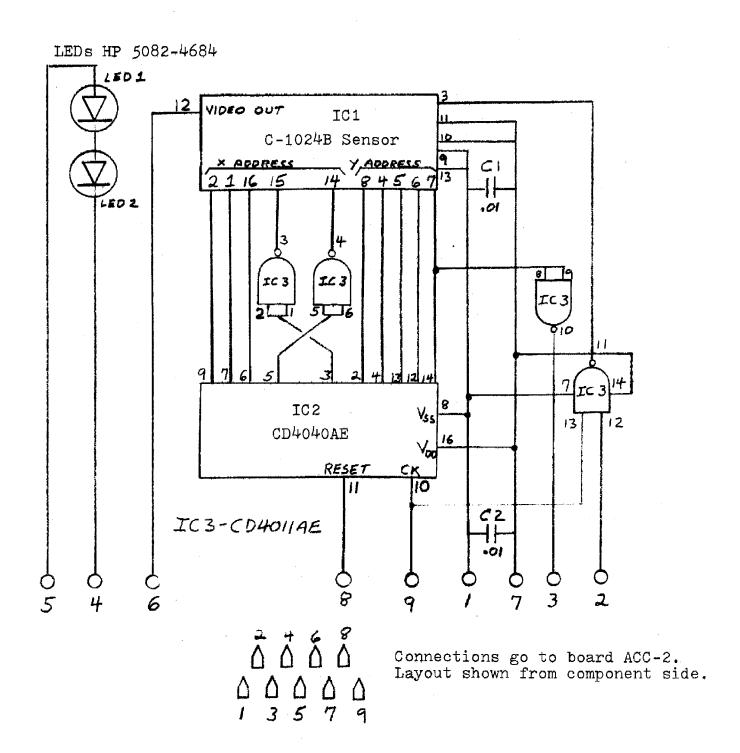
Schematic diagram of board ACC-1.
