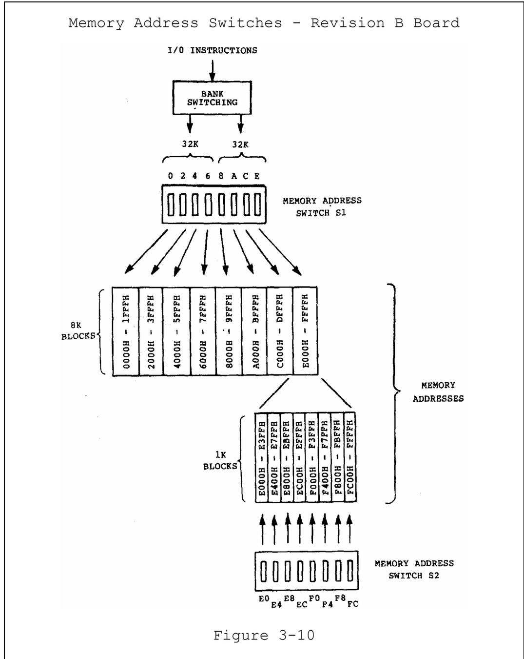
Each of the switches in S1 corresponds to one 8K section of the address space. The last 8K section is further divided into 1K sections by the switches in S2.
