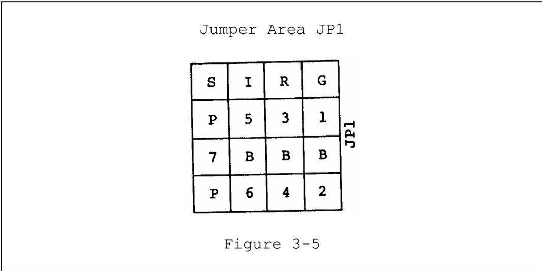
\*One of bits 5, 6, or 7 is used for parity error control, leaving a total of six bits that can be used for bank switching. Note that bit 0 is used to control the on/off function specified by the other seven bits.
