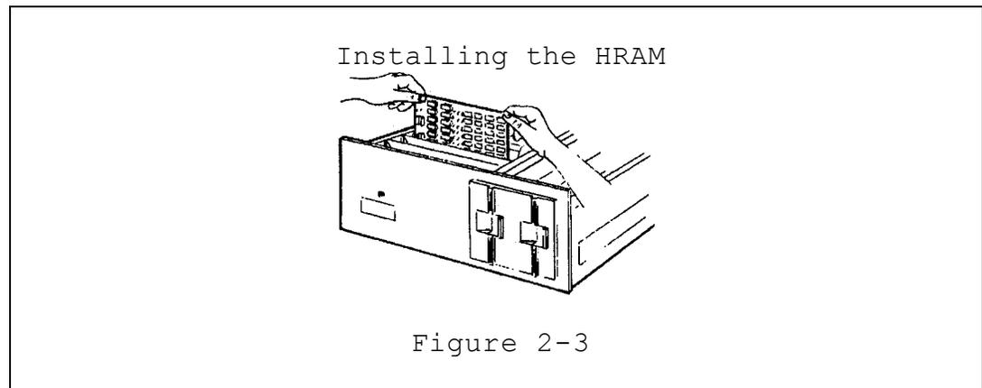
The row of metallic strips, or "fingers" on the bottom of the board should fit into the connector at the base of the card slot. Press firmly on the top of the memory board until the board is firmly seated in the connector.
