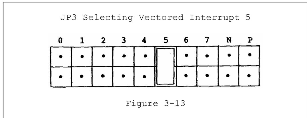
If you are using other software, you can pick another interrupt. NMI should only be used as an emergency service technique. If no interrupt is desired, the mini-jump can be stored by placing it sideways, as shown below.
