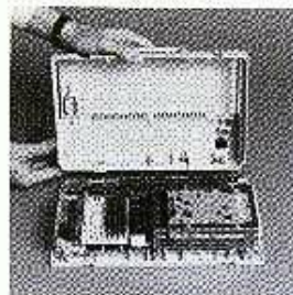
Figure 4-2 Removing the rear half of the case
