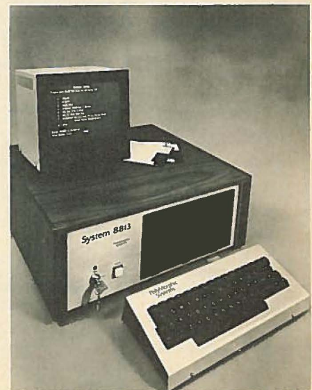
The minimum PolyMorphic 8813 system consists of one floppy disk (three are shown here) in the main cabinet, a typewriter keyboard, and a video monitor, plus 16K of RAM memory.
