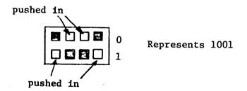
NOTE: (Some switches are marked ON/OFF; ON corresponds to a logic 0 and OFF to a logic 1.)
