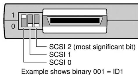
Figure 6-2 The SCSI ID Switch (Series 2 Drives only)
