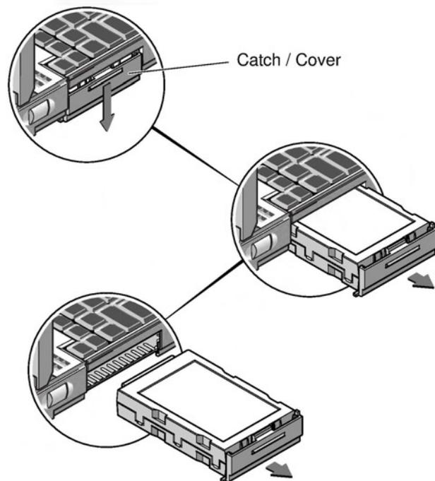
Figure 6-1 Removing the Hard Disk
