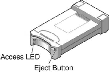
➤ To insert a floppy disk, hold it label side up and slide it into the aperture until it clicks into place.
