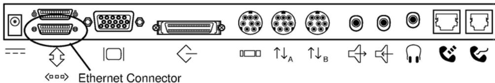
*Figure 8-1 Ethernet Connector*
