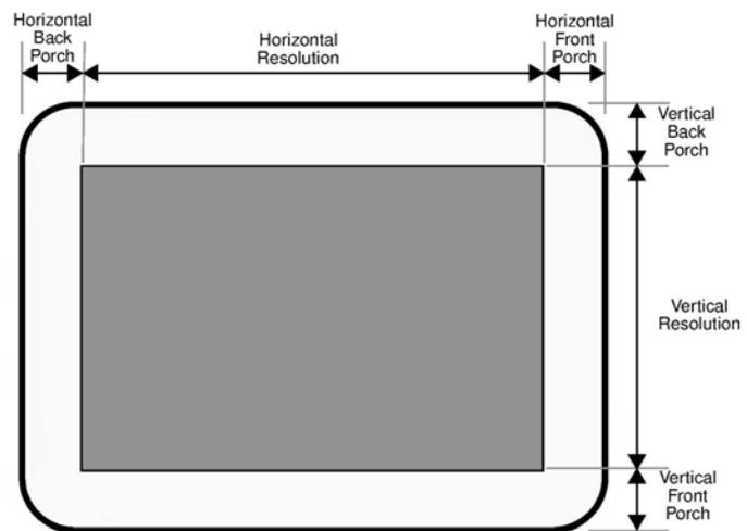
*Figure 11-7 Video Timing Parameters on the Displayed Image*
