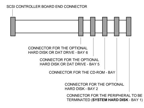
The following figure shows the simple connection of a SCSI controller to peripherals:
