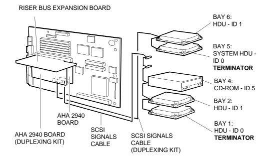
**Note:** In the duplexing configuration, the system hard disk (BOOT) must be the one connected to the second SCSI controller board installed in Riser bus slot 5 or 6.
