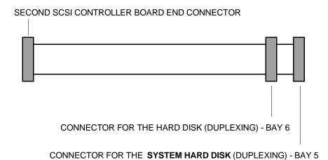
The following figure shows the connection of the two SCSI controllers used for the duplexing of hard disks:
