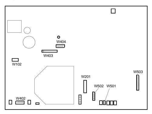
Fig. 28-7 Motherboard Connectors Location
