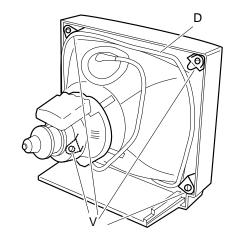
Fig. 28-9 Removing the CRT
