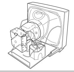
Fig. 28-4 Removing the Video Amplifier Board
