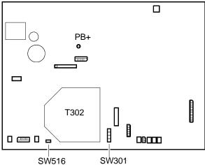
Fig. 28-14 Motherboard Adjustment Points
