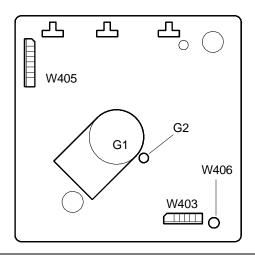
Fig. 28-5 Video Amplifier Board Connectors Location
