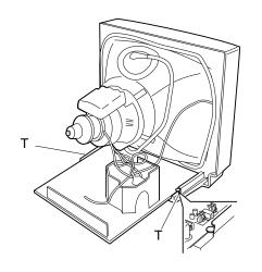
Fig. 28-6 Removing the Motherboard
