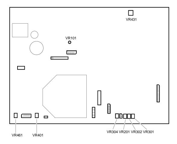
Fig. 28-13 Motherboard Adjustments
