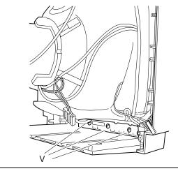
Fig. 28-8 Removing the External Controls Board
