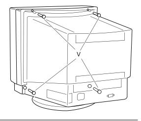
Fig. 28-1 Removal of Monitor Casing
