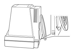
Fig. 28-2 Removal of the pedestal
