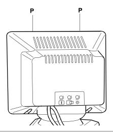
Fig. 35-3 Removing the Case of the Monitor - Locating Points P
