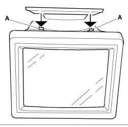
Fig. 35-1 Removing the Base
