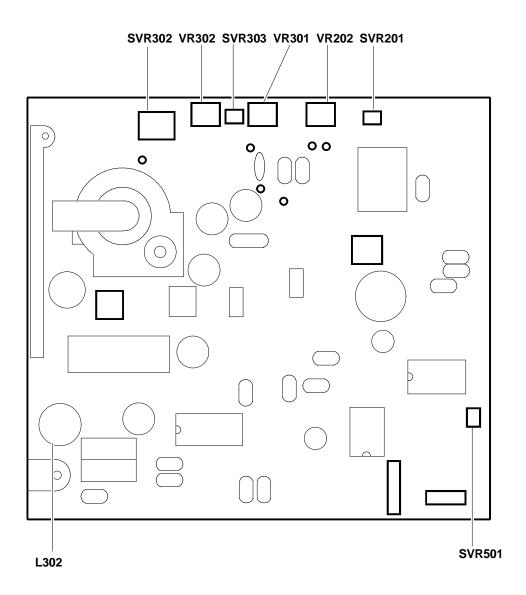
Fig. 35-15 Main Board Adjustments
