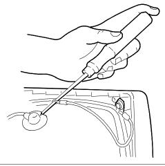
Fig. 35-4 Discharging the CRT Anode
