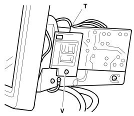
Fig. 35-8 Removing the ON/OFF Switch and Contrast Assembly
