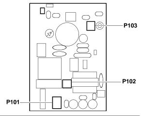
Fig. 35-6 Locating the Connectors on the Power Supply Board
