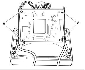
Fig. 35-9 Removing the Main Board
