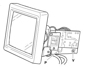
Fig. 35-5 Removing the Power Supply Board
