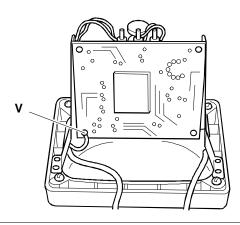
Fig. 35-7 Removing the Degaussing Cable Screw
