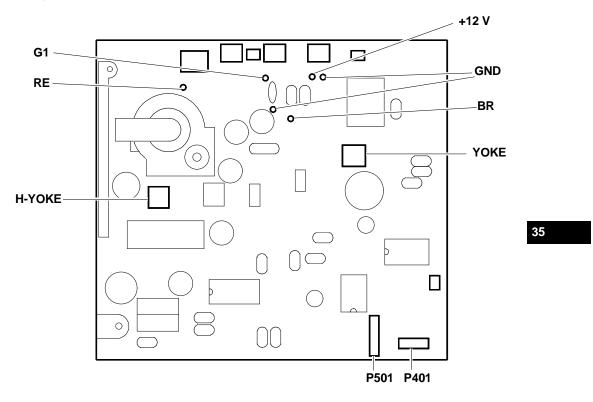
Fig. 35-10 Locating the Connectors on the Main Board
