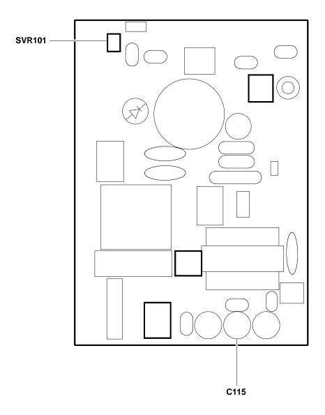
Fig. 35-14 Power Supply Board Adjustments
