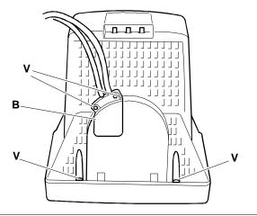
Fig. 35-2 Removing the Case of the Monitor
