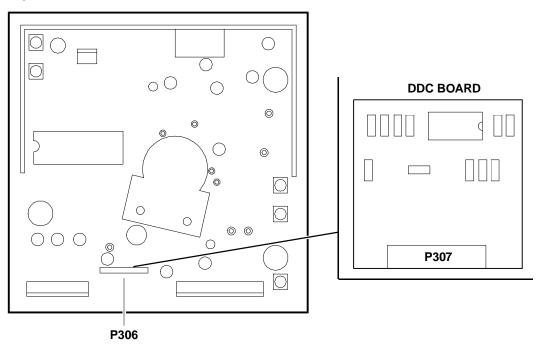
Fig. 37-2 Removing the DDC Board
