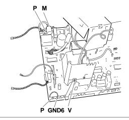
Fig. 39-9 Detaching the Main Board from its Metal Support
