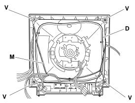
Fig. 39-11 Removing the CRT
