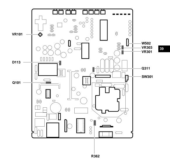
Fig. 39-14 Main Board Adjustments
