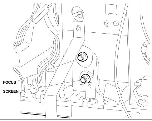
Fig. 39-16 Focus and Screen Potentiometers
