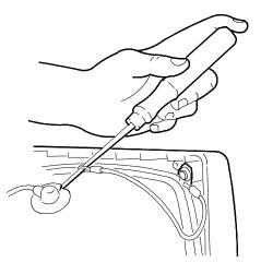
Fig. 39-4 Discharging the CRT Anode
