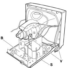
Fig. 39-7 Removing the Main Board
