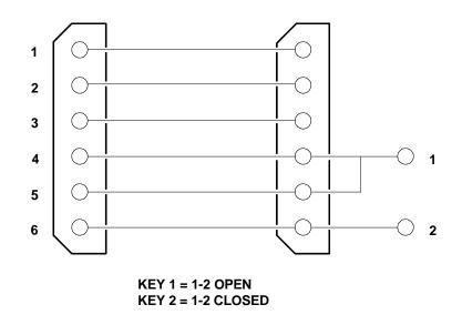
Fig. 39-15 JIG Adjustment Connector
