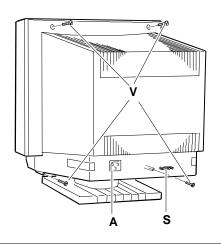
Fig. 39-2 Removing the Case
