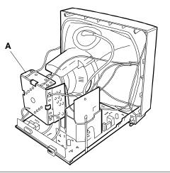
Fig. 39-5 Removing the Video Amplifier Board
