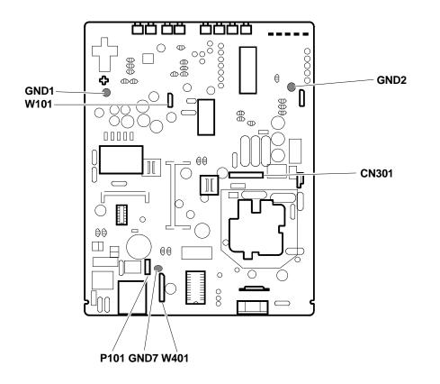
Fig. 39-8 Locating the Connectors on the Main Board
