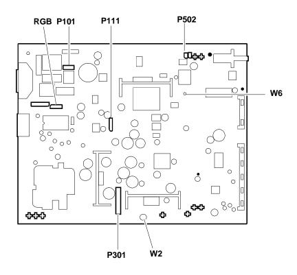
Fig. 42-8 Locating the Connectors on the Main Board
