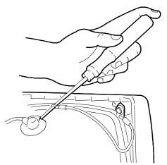
Fig. 42-4 Discharging the CRT Anode
