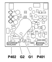
Fig. 42-6 Locating the Connectors on the Video Amplifier Board
