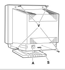
Fig. 42-2 Removing the Case
