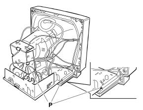
Fig. 42-7 Removing the Main Board
