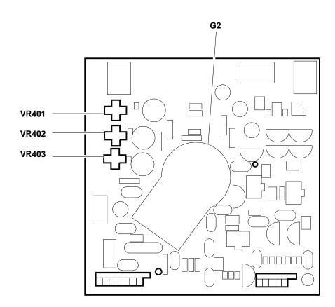
Fig. 42-13 Video Amplifier Board Adjustments
