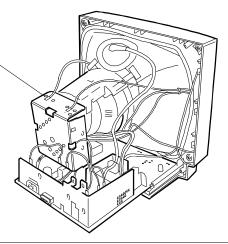
Fig. 42-5 Removing the Video Amplifier Board
