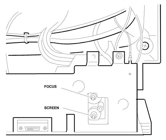
Fig. 42-14 Focus and Screen Potentiometers
