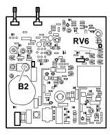
Fig. 5-5 - Horizontal linearity adjustment
