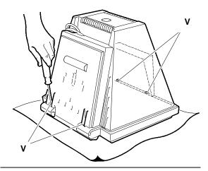
Fig. 5-1 Video casing screws positions
