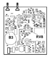
Fig. 5-6 - Horizontal width adjustment
