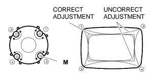
Fig. 5-10 Geometric distortion adjustment
