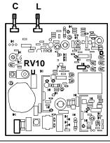
Fig. 5-3 Brightness pre-adjustment
