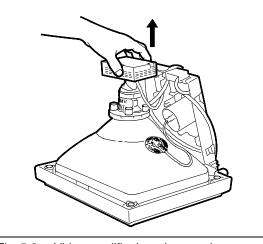
Fig. 5-2 Video amplifier board removal
