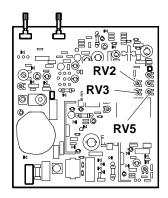
Fig. 5-7 Vertical width adjustment
