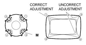
Fig. 6-10 Geometric distortion adjustment
