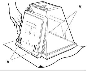
Fig. 6-1 Position of video casing screws
