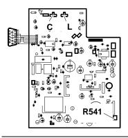
Fig. 6-4 Brightness pre-adjustment
