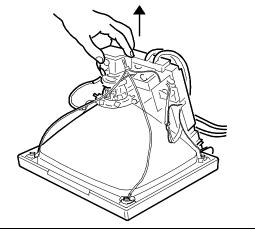
Fig. 6-2 Video pre-amplifier board removal
