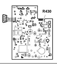
Fig. 6-5 Vertical linearity pre-adjustment
