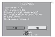
Select "Yes" to start downloading the firmware. When the firmware update starts after the downloading is finished, a black screen is displayed.
