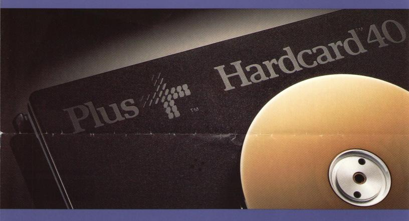
Hardcard<sup>™</sup> 40 is only one inch wide, enabling 42.26MB to fit easily into a single, full-length expansion slot in an IBM<sup>®</sup> PC,<sup>™</sup> XT<sup>™</sup> or AT<sup>™</sup> without compromising adjacent slots.
