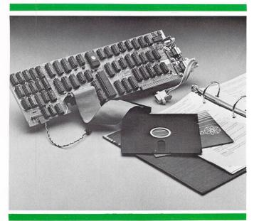
The Quadlink package: hardware, software, and user's guide
