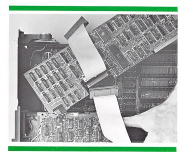
Attach the disk controller cable into the lower rim of gold fingers located near the middle of the board. Make sure the connection is snug and the pin numbers on both connection points match.
