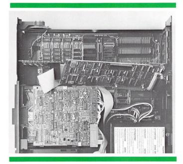
Attach the Quadlink's disk controller cable to the left edge connector of the system's disk controller card. Again, make sure the pin line ups match as the connection is made. Then insert the disk controller card into expansion slot #5.
