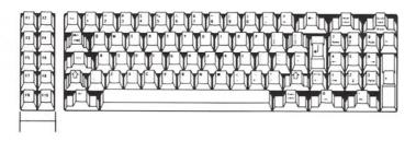
In the IBM mode, the function keys perform certain programmable operations that replace CONTROL commands issued from the standard keypad. The function keys serve as a shortcut to initiating these commands. For instance, when using IBM BASIC, the F2 key gives the RUN command when pressed, saving you from having to type another line into you program.
