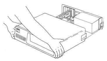
Pull the cover off until the inside circuitry is exposed.
