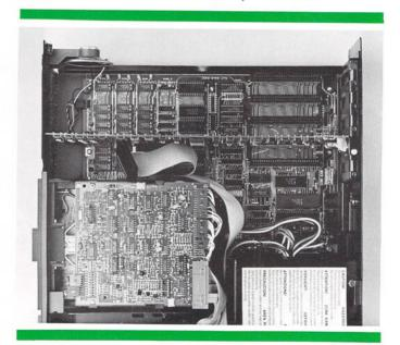
Snap the Quadlink's right rim of gold fingers down into expansion slot #4 on the system mother board. The board can then be secured in place by screwing the cover plate down into the top of the chassis.
