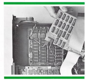
Detach the speaker wire from the mother board connector and reroute the wire to connect it into the left-most gold pins located on the lower left corner of the board, next to the Quadlink's installed speaker wire.
