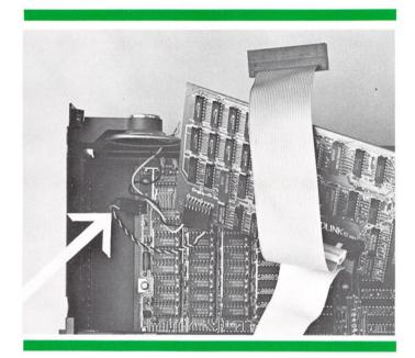
Take the free end of the Quadlink's speaker wire and insert it into the mother board connector. When this is done the speaker will be wired through the Quadlink back to the mother board.
