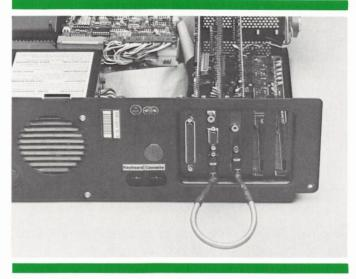
Take the video cable and attach one of the female nine-pin sub mini D-type connectors into the lower nine-pin connector on the Quadlink end plate. Take the other end and connect it into the nine-pin connector on the video display card.
