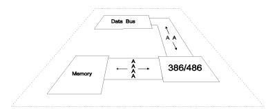
In view of the above, you can see that processor speed alone is no guide to performance, and in some cases may even be irrelevant. A slow hard disk (on the data bus), for instance, will always make any processor wait for its data and waste cycles that could be used for serious work. In fact, as far as NetWare is concerned, a 486/33 is only noticeably better than a 386 when network loading is heavy (the same goes for later chips, I'm sure).
