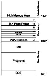
DOS was written to run applications inside the bottom 640K block simply because the designers of the original IBM PC decided to - memory then was expensive, and most CP/M machines only used 64K anyway (the PC with 128K was \$10,000!). Other machines of the same era used more; the Sirius allowed 896K for programs.
