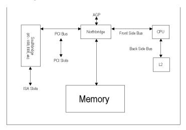
Essentially, the functionality of the chipset is combined on two main components, the Northand South- Bridge chips, which live at each end of the PCI bus. The CPU, Memory and AGP talk to the Northbridge and the Southbridge handles all the I/O, including the ISA bus. NVidia calls them the IGP and MCP, respectively, standing for *Integrated Graphics Processor* and *Media and Communication Processor* (their chipset also uses AMD's Hypertransport technology, which is mentioned below).
